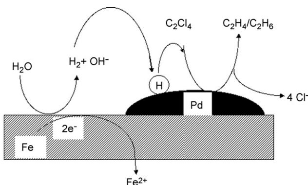
Fig. 7. A conceptual model for the hydrodechlorination of tetrachloroethylene. Atomic hydrogen is expressed as  $\text{H}$ .
