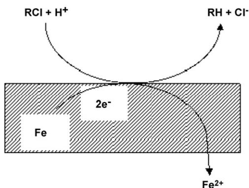
Fig. 1. Depiction of the ZVI-mediated degradation mechanism: the direct reduction model. RCl and RH represent chlorinated hydrocarbons and hydrocarbons, respectively.
