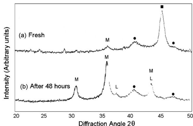
Fig. 4. Comparison of XRD spectra of nanoscale Pd/Fe particles with 5% palladium before and after reactions with TCE. Solid square and circle represent Fe(0) and Pd(0), respectively. Iron oxides include magnetite/maghemite ( $\text{Fe}_3\text{O}_4/\gamma\text{-Fe}_2\text{O}_3$ ) (M) and lepidocrocite ( $\gamma\text{-FeOOH}$ ) (L).
