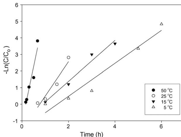
Fig. 5. A plot of  $\ln(C/C_0)$  vs. time for the reduction of PCE by nanoscale Pd/Fe particles.
