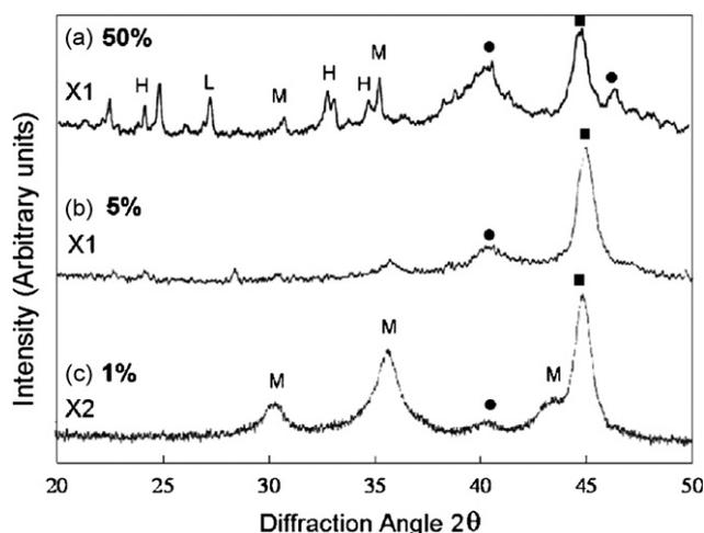
Fig. 3. XRD spectra of nanoscale Pd/Fe particles with different palladium contents. Solid square and circle represent Fe(0) and Pd(0), respectively. Iron oxides include magnetite/maghemite ( $\text{Fe}_3\text{O}_4/\gamma\text{-Fe}_2\text{O}_3$ ) (M), hematite ( $\alpha\text{-Fe}_2\text{O}_3$ ) and lepidocrocite ( $\gamma\text{-FeOOH}$ ) (L).
