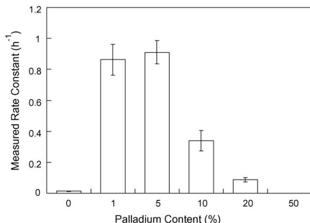
Fig. 2. Rate constant for the reduction of TCE by Pd/Fe bimetallic particles as a function of the palladium content. The initial TCE concentration was 120 mg/L and nanoparticle loading was 5 g/L.
